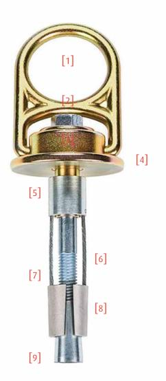
The Hybrid MEGA Swivel Anchors utilize combined technology of MEGA Swivel and Concrete Anchors. The patent pending key lock design keeps the D-ring seated and locked into its swivel housing, preventing the steel from spreading outward during heavy loads.
