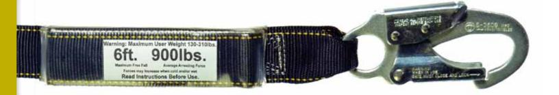
• **3.1.8.1** 6 ft. free fall personal energy absorbers and energy absorbing lanyards when tested in accordance with 4.4 and 4.5 shall have an average arrest force no greater than 900 pounds and a maximum deployment distance of 48 inches without exceeding 1,800 pounds maximum arrest force.
